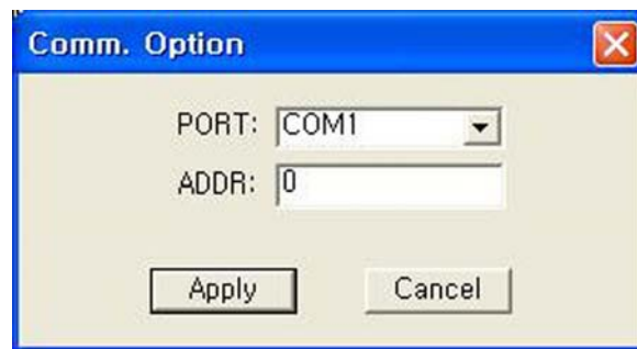
<Figure 15. Communication Port Configuration>
