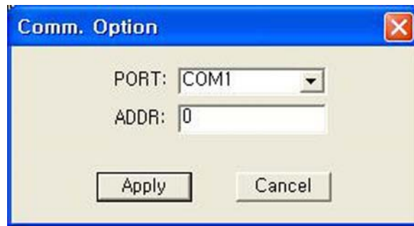
<Figure 13. Communication Port Configuration>
