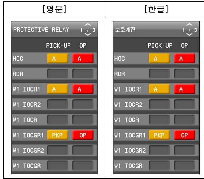
<Figure. PROTECTIVE RELAY 상태 화면>
